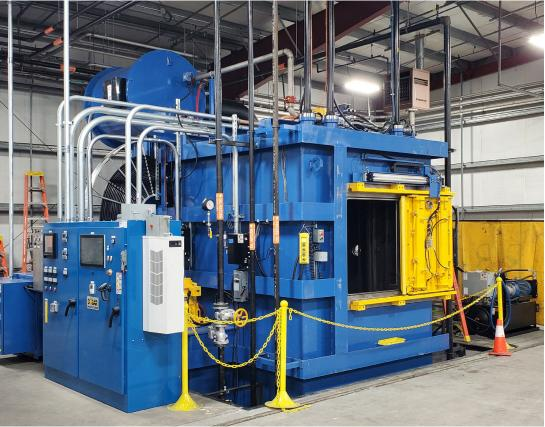
new furnace is **SAFETY**. A tightly sealed vacuum chamber with a fully purged nitrogen vestibule eliminates the need for traditional burn off ports or flame curtains because endothermic protective atmospheres are no longer needed. Additionally, detrimental CO2 gas emissions to our atmosphere will be reduced dramatically. These features alone will provide a safety culture boost to our oftenmaligned heat treating industry.
