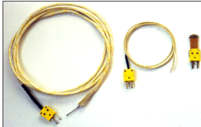
Thermocouples (thermoelectric couple- Seebek Effect)
