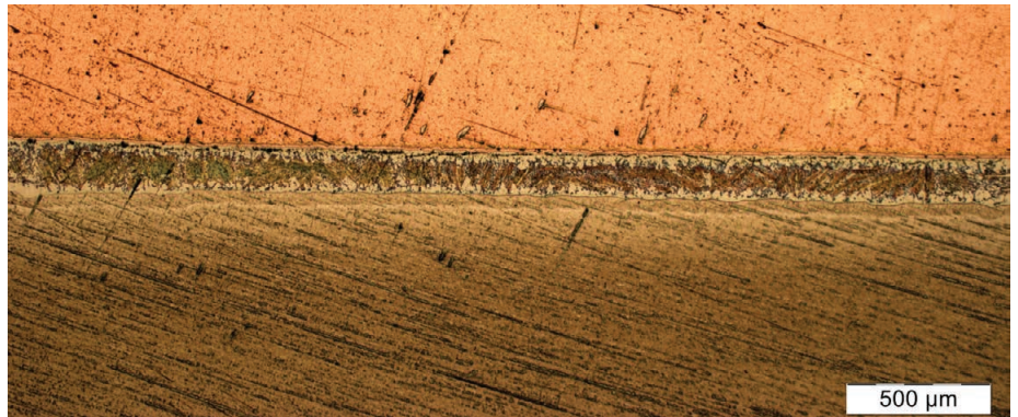
Fig. 2 Titanium Grade 2 brazed to copper using amorphous foil TiBraz800 at 830°C
