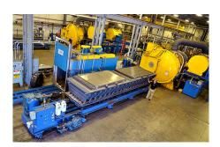
retention screens that were 80-inch-wide, we needed to take advantage of the 84-inch-wide potential in the furnace. *Read more...*
