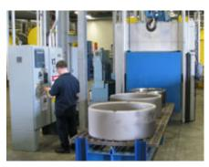
A new air furnace at Solar Atmospheres of Western PA is speeding delivery time and providing more vacuum processing capacity for our customers. This large, electric re-circulating air furnace works in conjunction with our vacuum furnaces to improve customer service.
