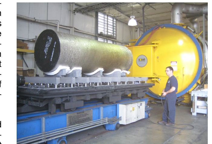
15,000 lb. ingot before homogenizing
