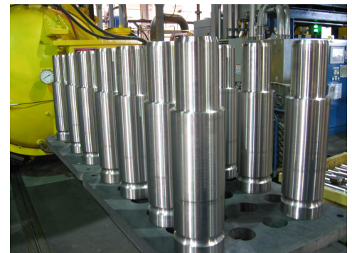
Large Load of 4340 for vacuum carburizing
