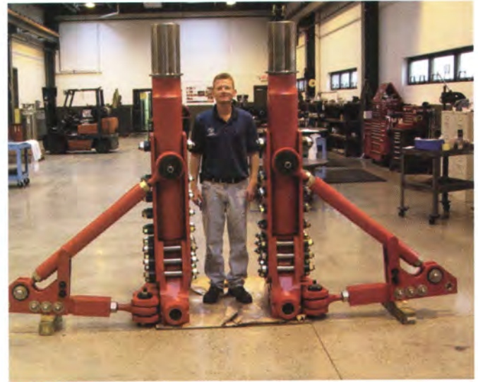
Landing gear with vacuum heat treated 4340 and 4340M components
