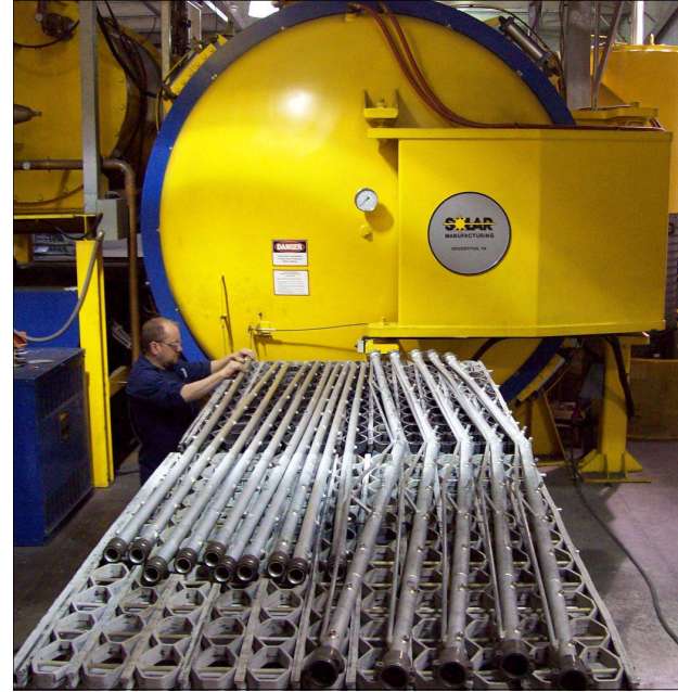
Tubes of aluminum prepare to be vacuum heat treated
