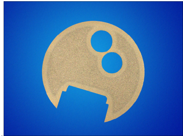
10X magnification of vacuum carburized case on part cross section
