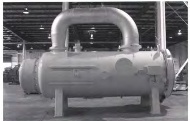
New carburizing furnace on the floor at Solar Atmospheres.
