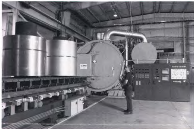
50,000 lb. load on Solar's newly patented "transfer system"
