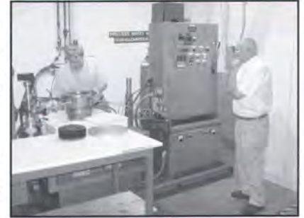
Bill and Trevor Jones operate the experimental vacuum carburization furnace built at Solar.
