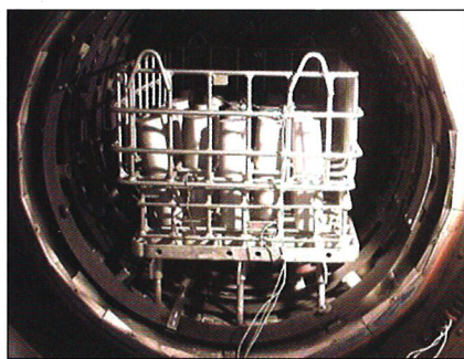
Fig 4 Test loads used to determine improvements of quenching using higher gas velocities
