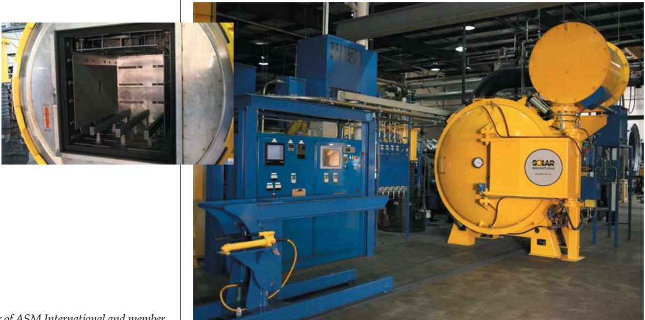
**Fig. 1 — Vacuum furnace and control system.**
