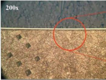
Fig. 8 — Cross section of vacuum gas-nitrided surface.
