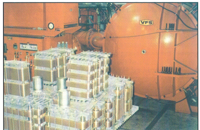
Fig. 4 Heat exchangers after copper braze cycle.
