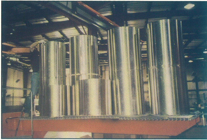
Fig. 5 Mumetal and Carpenter 42 alloys after hydrogen magnetic anneal.
