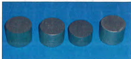
Fig. 10 — One control sample and 3 preoxidized samples nitrided after preheating in H 2 to a temperature of 524°C and 125 torr; (top) before entering furnace; (bottom) after nitriding.
