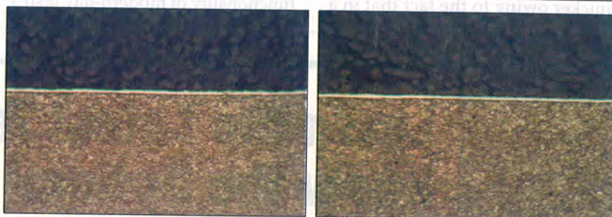
Fig. 12 — Photomicrographs of test samples nitrided at 524°C and 812 torr in preoxidation test B; (left) control: no preoxidation; (right) preoxidized at 427°C. Magnification: 200×
