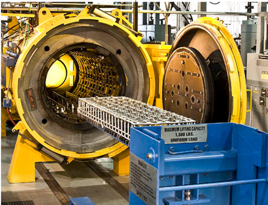
Gears ready for heat treating in a vacuum furnace.
