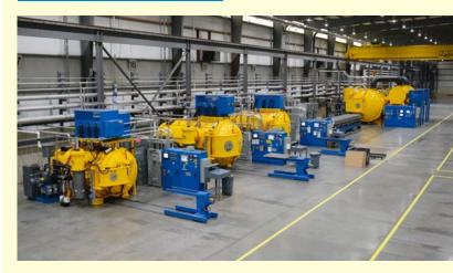
Solar Atmospheres newest facility in Greenville, South Carolina has a wide range of vacuum processing capacity now available. From furnaces suited for small lots and development cycles to a 24 foot long vacuum chamber capable of processing up to 50,000 lbs at 2650°F. All backed by AS9100 and Nadcap quality systems to provide the assurance that your product is being processed as it should be.
